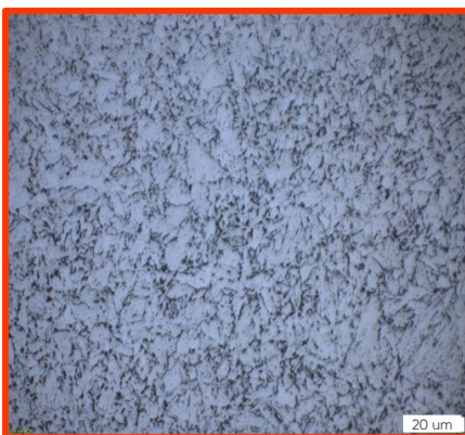
Ref1857 and 1858 (µ): after cycle A +cycle B1 (720°C/180s +WQ)
